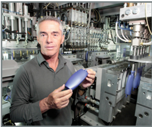
Techne SpA CEO and owner Moreno Minghetti shows the inner workings of the company's high-output Advance blow molding machine, which the company bills as an alternative to long-stroke machines. (Joe Wilssens photo)
